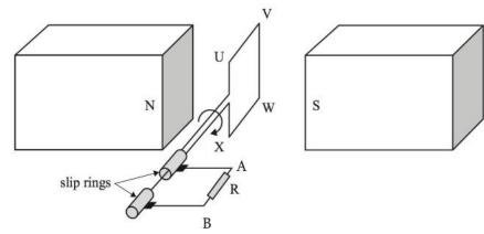
(a) Calculate the peak voltage  $(\mathcal{E}_{max})$  of the generator.
